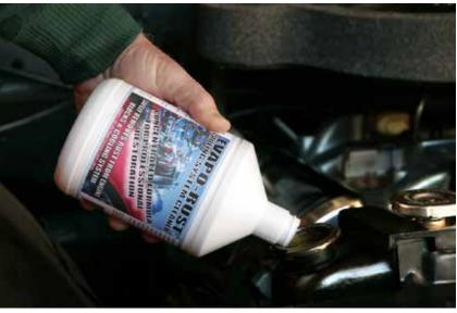
EVAPO-RUST Cooling System Cleaner is a concentrated rust removing formulation based on our 3-TIME AWARD WINNING rust remover technology. Cooling System Cleaner works through selective chelation at a pH of 6.1 to 7.0 (neutral) and does not require any special equipment or personal protective wear.
