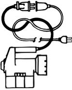
If you need a longer power cord, we recommend a garden-type extension cord. Do not use one that is cut, frayed or otherwise damaged. To prevent accidental unplugging, knot the two cords as shown, or use a cord retainer available at many hardware stores at modest cost.
